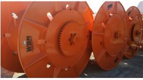
The WBM Cable Reeler CR200/300 Series are designed to safely and efficiently handle the distribution and trailing cables for electric powered equipment in underground or open pit mines.
