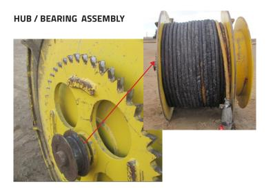
Bull gear drive – engages with the pinion drive gear on the reeler frame
