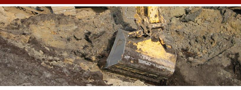
The TCB Twist-a-Bucket and Chuck Blade combination is designed to increase machine versatility. Remove three pins to change your attachment to suit the job. Choose between our rugged Chuck Blade or the versatile Twist-a-Bucket.
