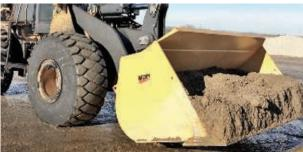
WBM's Spreader Bucket is an excellent dual purpose attachment that is designed to easily spread sand/small aggregate on roadways and can be used as a regular general purpose bucket as well.
