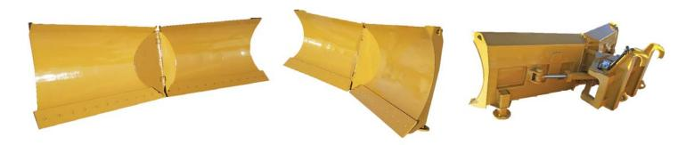
The WBM U/V Angle Blade is the most versatile blade available for a motor grader. It is capable of operating as a straight blade, angle blade, u-blade or v-plow. It is used extensively for snow removal and is extremely useful due to its functionality. Auxiliary hydraulics are utilized along with an optional diverter valve to enable operator controlled blade changes between all four configurations. The U/V Angling Blade is available in either KAT Master Hitch or Integral Lift Group designs.
