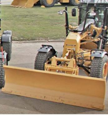
WBM Motor Grader Snow Blades are designed with an effective curvature that increases capacity and allows the 'rolling' action required to efficiently clear snow with ease.
