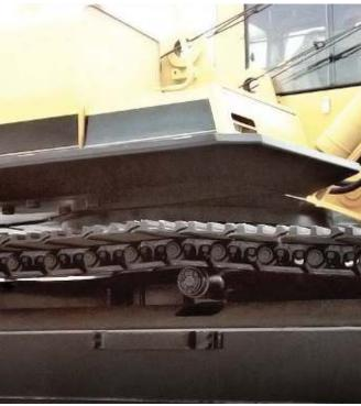
WBM Underhouse Guards are used primarily in harsh environments (ie: forestry) to protect the underside of the excavator from protruding and harmful objects.
