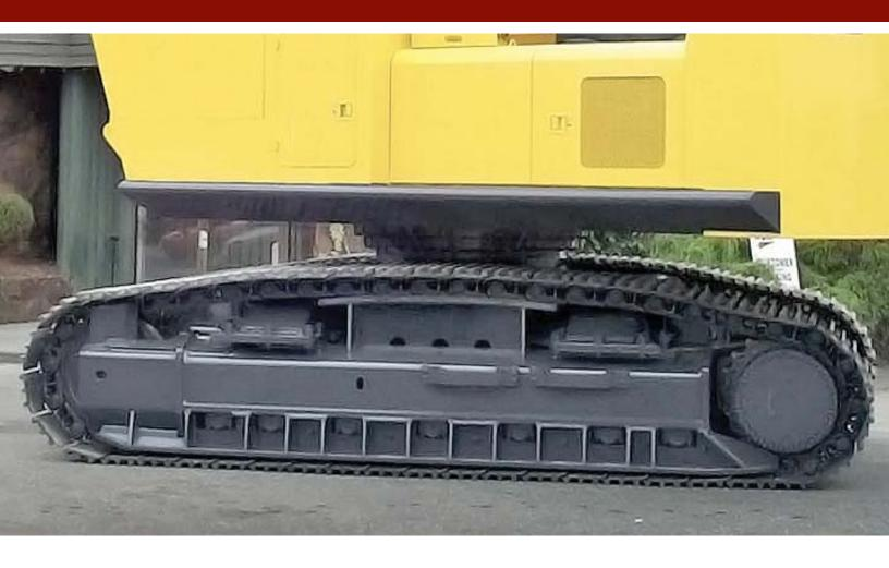
WBM Rock Guards protect the excavator track from foreign objects and debris. They are used in environments where track damage is common (ie: forestry, road building and demolition). Rock Guards also provide an excavator with pad support when being used in a rocky or unstable environments.
