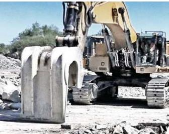
WBM Concrete Removal Buckets are designed to effectively handle slabs of concrete.
