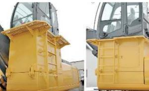
WBM Cab Risers are used primarily in forestry and road building applications.
