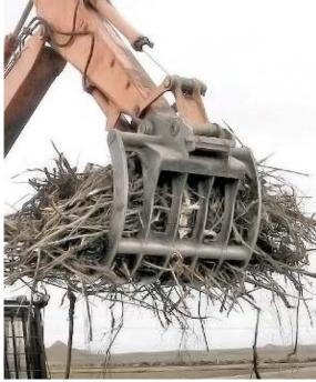
The WBM Brush Rake is primarily used in the forestry and road construction industries to remove and pile brush, roots and stumps without retaining soil.
