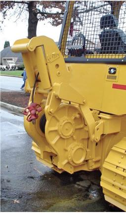
WBM Designed & Built Arches have been proven in rugged logging country and are adapted to a wide variety of special winching applications. Four roller configuration permits maximum line pull from all angles with minimum cable wear.
