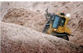
WBM's Chip Blade is used primarily in the Pulp and Paper industry for the stockpiling of wood chips. These high capacity U-blades are designed to increase productivity through efficient moldboard curvature and improved carrying capability and match machine specifications.
